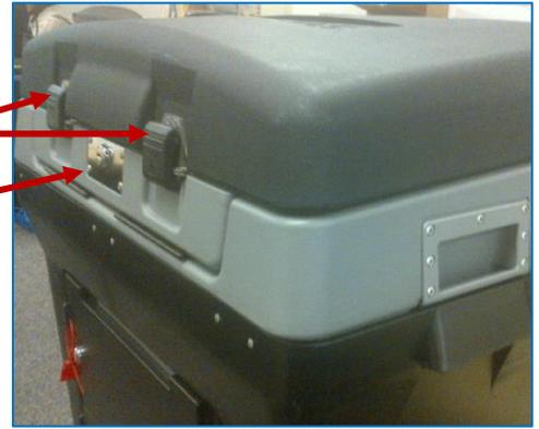
Use the silver key to open access panel on the back of tabulator. Carefully remove electrical cord. Plug electrical cord into a three-prong grounded outlet.
