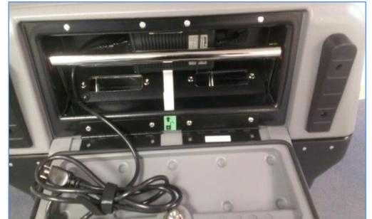
After plugging in the tabulator, use the barrel key to unlock scanner and gently lift screen to open. Do not close screen until the polls have closed. The DS200 will begin booting up.
