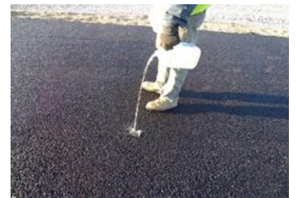
Water quickly infiltrates through porous pavement.
