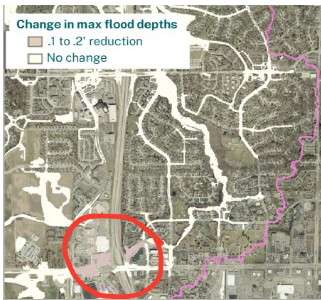
Figure 4 Hypothetical modeling removed all runoff on Menards from model. The result is small reductions in flood depths around Mineral Point Road and Target pond in 1% chance storm. By the time the water reaches the Sauk Creek greenway, there are no changes in flood depth.
