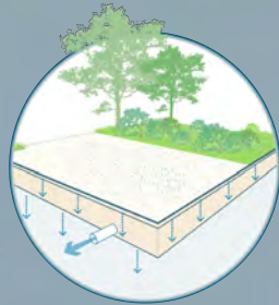
Pervious Paving Rain water that falls within the pavers will make its way back into the ground through an underground layer of stone.
