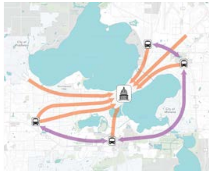
Figure 9: Madison's geography and development pattern drives a radial (orange arrows) network design. A ring of orbital routes (purple arrows) connect with the radial services.
