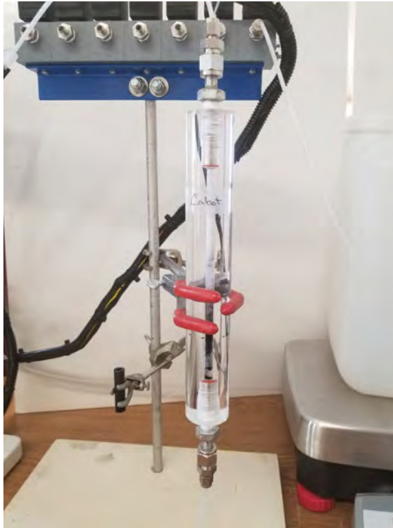
Figure 3: RSSCT column loaded with Cabot Norit GAC 1240 Plus
