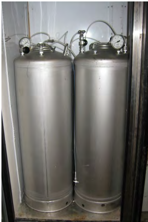
Figure 1: Stainless steel holding tanks for RSSCT influent
